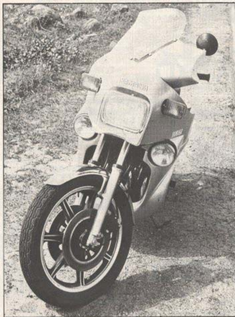
Mockett's strange fairing is surprisingly slim. Note handlebar and screen section rotates with steering head while the rest of the structure is firmly fixed to the frame.
